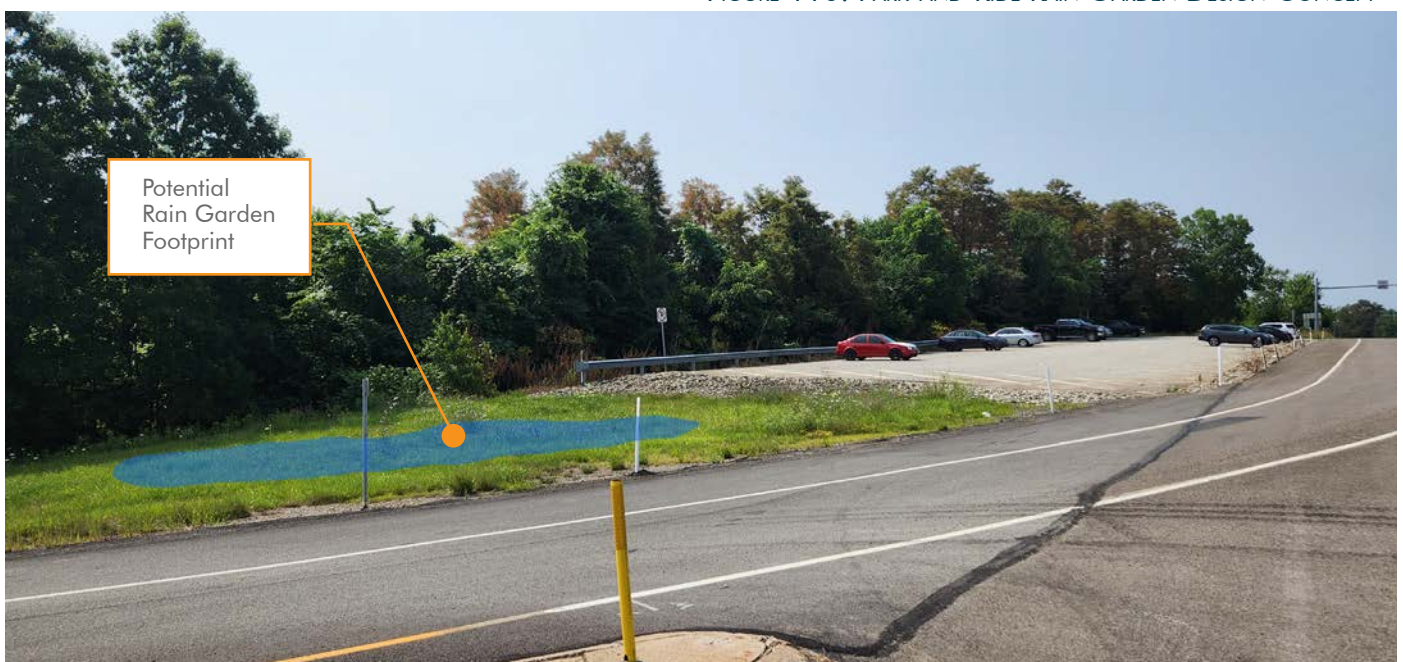
FIGURE 110: PARK-AND-RIDE RAIN GARDEN DESIGN CONCEPT
